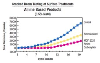
MCI-2020 reduced corrosion current by 72% compared to the untreated sample, and also outperformed the aminoalcohol based surface treatment.
